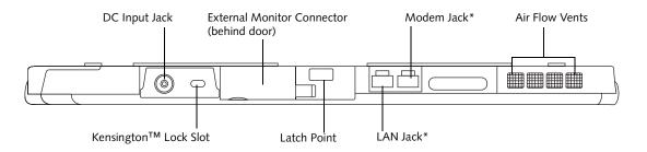
Figure 1-5 Stylistic ST4000P Series Pen Tablet PC Features (Left Side View)
